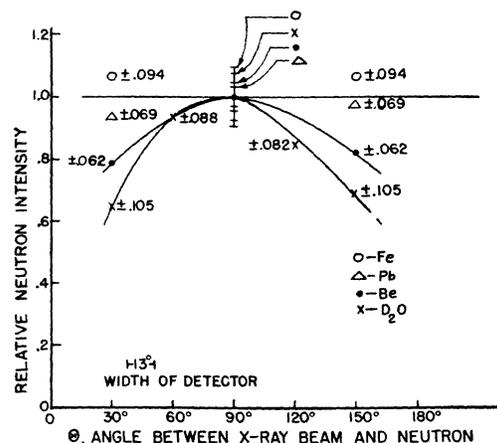
FIG. 3. Angular distributions of photo-neutrons for bremsstrahlung spectrum with maximum energy of 19.7 Mev. Intensities are normalized at  $90^\circ$  and probable errors are given for each point.
