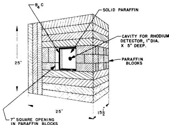
FIG. 1. Fast neutron detector. The front plate, which is made of Lucite and boron carbide, has been removed to show the location of the rhodium detector.
