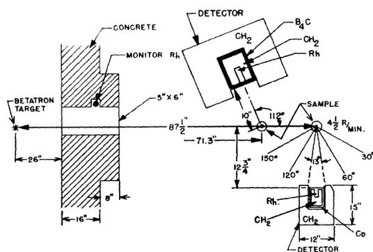
FIG. 2. Schematic diagram of apparatus. During measurements only one detector was in position at any time.
