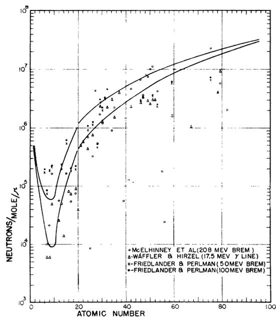
FIG. 5. Comparison of photo-neutron yields. Solid curves indicate results by Kerst and Price. The yields measured by McElhinney *et al.* are absolute whereas those measured by Wäffler and Hirzel, and Friedlander and Perlman are relative and have been normalized at  $Z=47$ .
