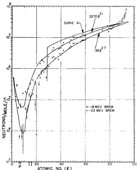
FIG. 4. Yields of photo-neutron sources for two bremsstrahlung spectra. Probable errors are shown by vertical lines through each point. Curve  $A$  is the yield predicted by Goldhaber and Teller which has been corrected for the 22-Mev bremsstrahlung spectrum and normalized at  $Z=90$ . The observed yield at  $Z=29$  is about half the predicted yield because approximately half of the resonance is below 22 Mev.
