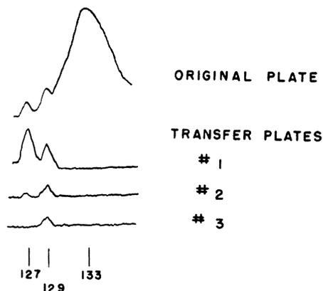
FIG. 4. Microphotometer tracings of mass spectrograph plates. Transfer plate 1 was exposed to the original plate, emulsion to emulsion, immediately after removal from the mass spectrograph, and remained on for 24 hr. Transfer 2 was exposed for the next 48 hr. Then transfer 3 was exposed approximately the next 72 hr.
