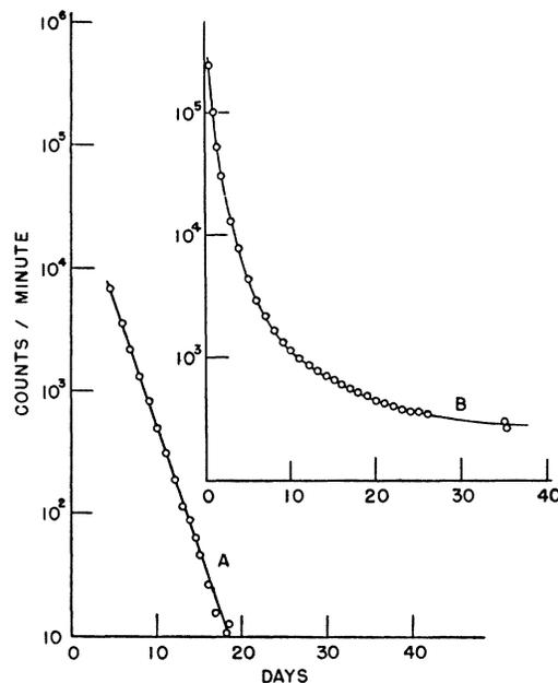
Fig. 3. Effect of re purification. Decay curve A is for a sample from which xenon was expelled by boiling from a solution after the 5.5-hr. cesium was effectively dead. Curve B is for a cesium sample which was not disturbed.
