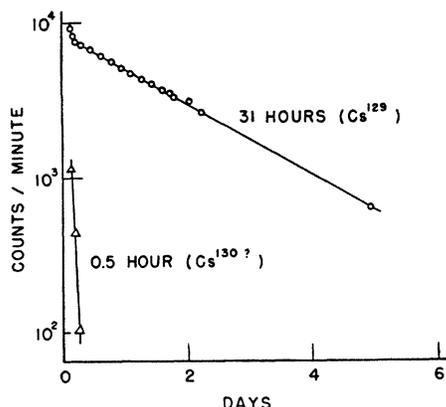
Fig. 2. Decay curve of cesium radioactivities induced from ammonium iodide by 36-Mev helium ions.
