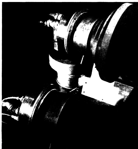
FIG. 5. Fission chambers and absorbers used in "poor geometry" measurements.
