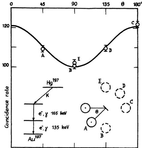
FIG. 1. Angular variation of coincidence rate of successive *L*-electrons from Au<sup>197</sup>.
