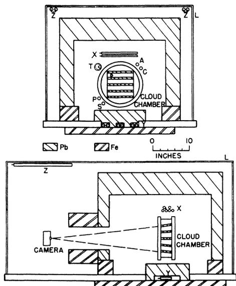
FIG. 1. Two perpendicular sections showing the disposition of absorber and counters about the cloud chamber. The chamber is triggered by various coincidences in the counters at X, Y, and Z.
