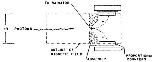
FIG. 2. Plan view of pair counters.
