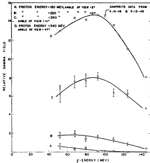
FIG. 4b. Relative gamma-yield from  $\frac{1}{2}$ -in. carbon target at various proton energies.
