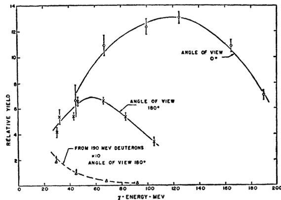
FIG. 3. Relative gamma-yield vs. energy from 2-in. Be target, bombarded with 350-Mev protons.
