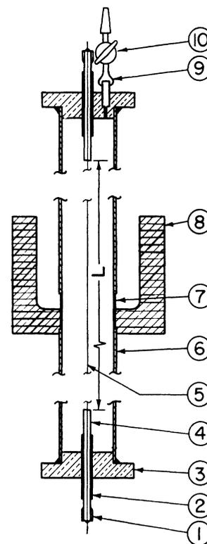
FIG. 1. Cross section of counter. 1—Brass cap. 2— $\frac{1}{8}$ -in. Trubore Pyrex tubing insulator. 3—Brass end plug. 4— $\frac{1}{8}$ -in. O.D. Kovar shield. 5—0.005-in. Kovar wire. 6—Brass shell, 1 in. O.D., 0.035-in. wall thickness. 7—Wall thickness 0.010 in. in this region. 8—Micarta refrigeration well. 9—Kovar to glass seal. 10—Stopcock and 10/30 standard taper ground glass joint.
