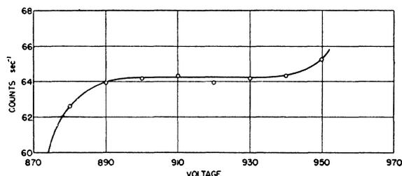
FIG. 2. Counting rate versus voltage characteristic for Geiger tube at  $\text{CO}_2$  partial pressure of about 2 mm Hg and total pressure 10.0 cm Hg.
