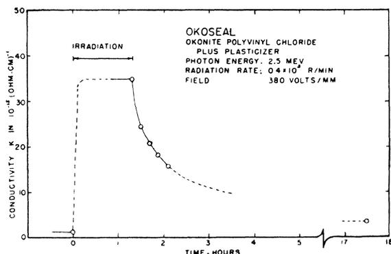
FIG. 1. Conductivity of Okoseal showing effect of irradiation.
