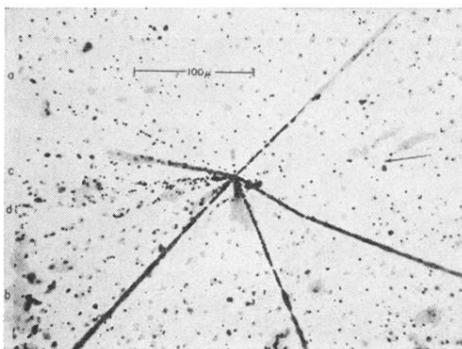
FIG. 2. Disintegration with 12 heavy prongs, 12 min. and near-min. tracks within  $100^\circ$ . Between *a* and *b*,  $52^\circ$  apart, are 8, and between *c* and *d*,  $10^\circ$  apart, are 5 minimum ionization tracks.
