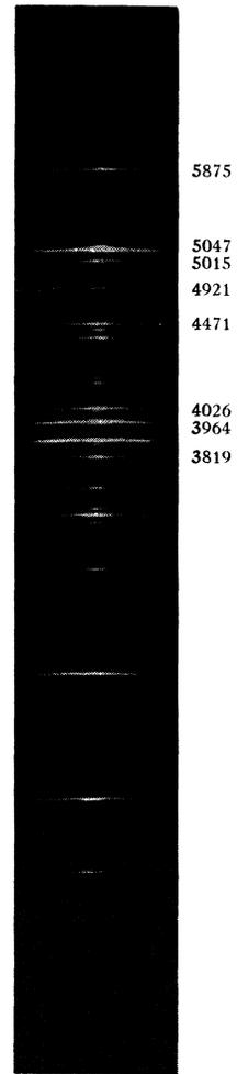
FIG. 8. Spectrogram of the glow around an electron beam projected between metallic electrodes. 100 volts accelerating potential; 0.06 mm pressure.
