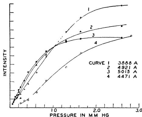
FIG. 2. Abundance curves for four characteristic transitions in the middle pressure region. Tube potential 70 volts; tube current 50 milliamperes.
