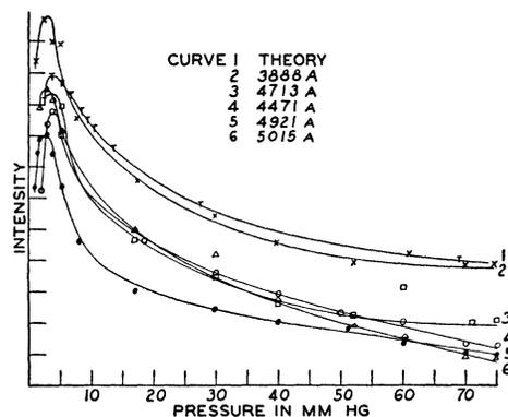
FIG. 3. Abundance curves for five characteristic transitions in the high pressure region. Tube potential 50 volts; tube current 30 milliamperes.
