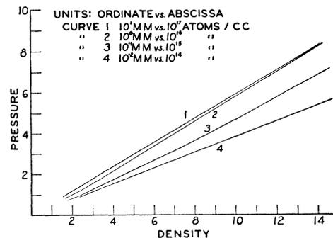
FIG. 5. Density (in atoms per cc) versus gas pressure in millimeters. For use with Figs. 1-4. The densities have been computed by the use of gas temperatures measured under operating conditions.
