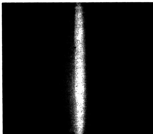
FIG. 10. Same condition as Fig. 9, except for 300 volts potential applied between deflector plates. Notice asymmetry of beam.
