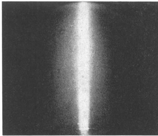
FIG. 9. Photograph, using green filter, of the 5875Å glow about a beam passing between metallic plates. The accelerating potential on the beam has been increased to 100 volts.
