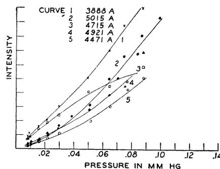
FIG. 1. Abundance curves for five characteristic transitions in the low pressure region. Tube potential 70 volt; tube current 50 milliamperes.
