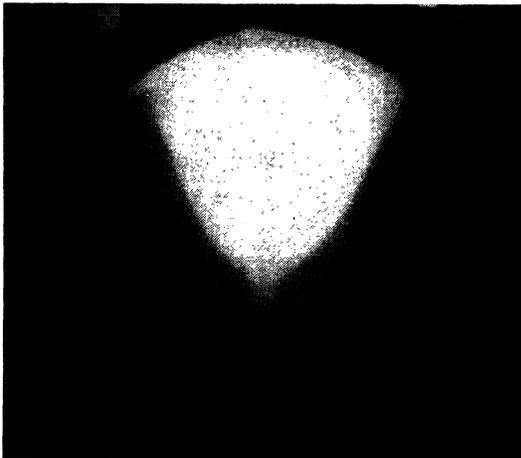
FIG. 7. Radiation produced in helium by an electron beam projected between metal plates, in comparison with Fig. 6, the influence of the electrodes on the contour of the discharge can be seen. 0.04 mm pressure; 60 volts accelerating potential.
