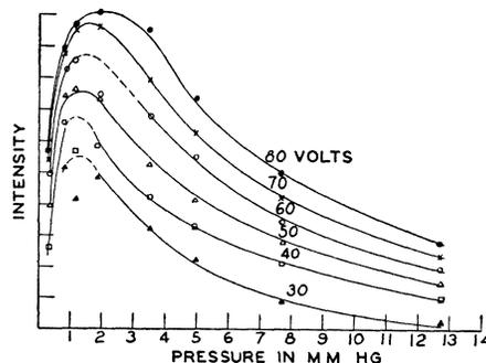
FIG. 4. A family of abundance curves at various tube potentials for the 5015 Å line of helium; 10 milliamperes tube current.
