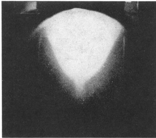
FIG. 7. Radiation produced in helium by an electron beam projected between metal plates, in comparison with Fig. 6, the influence of the electrodes on the contour of the discharge can be seen. 0.04 mm pressure; 60 volts accelerating potential.
