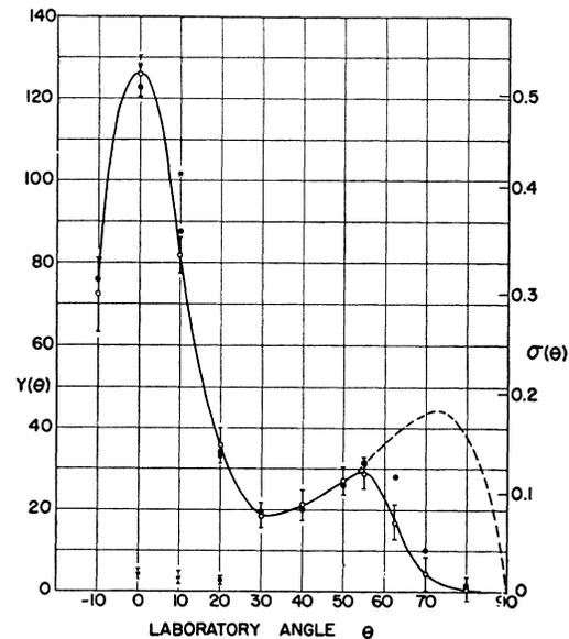
FIG. 2. Coincidence counting data as a function of laboratory angle  $\theta$  for recoil deuteron.  $Y(\theta)$  = net number of coincidence counts per 64,000 alpha-monitor counts.  $\sigma(\theta)$  = cross section per unit solid angle. The dashed curve is an extrapolation drawn to give an area under the curve corresponding to the total scattering cross-section value taken from reference 10.
