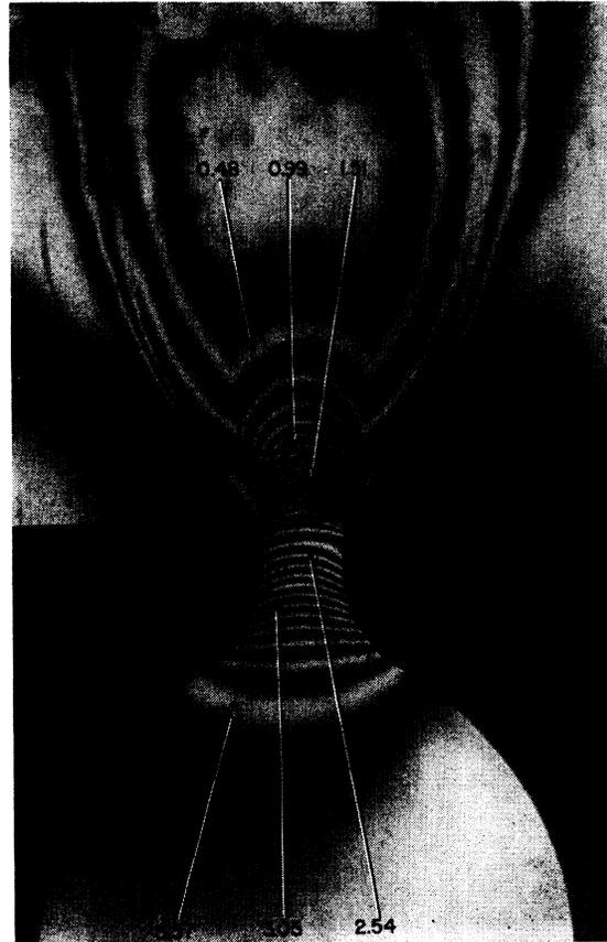
FIG. 20. Interferogram of contour fringes for two-dimensional jet flowing upward from reservoir through nozzle, fringes labeled in  $\text{mg}/\text{cm}^3$ . Expansion ratio 9.7:1.
