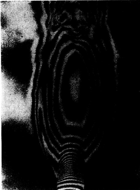
FIG. 19. Interferogram of contour fringes for two-dimensional jet, expansion ratio 6.1:1.
