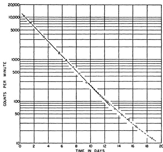
FIG. 1. Decay of separated lanthanum. Half-period is 41 hours when allowance of 10 counts per minute (i.e., 0.1 percent of initial activity) is made for barium contamination.
