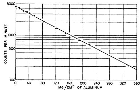
FIG. 2. Absorption of  $\beta$ -rays of  $\text{La}^{140}$  in aluminum. Crosses refer to lanthanum extracted from irradiated barium, circles to spectroscopically pure lanthanum after irradiation in the pile.
