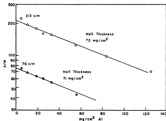
FIG. 1. Absorption curves taken on KCl samples. Upper curve: after neutron irradiation and subsequent purification from radioactive species other than  $K^{40}$ . Lower curve: KCl which was not irradiated.
