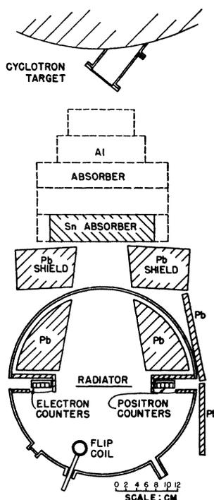
FIG. 1. Geometrical arrangement of the spectrometer, the absorber, and the cyclotron target. The actual positions occupied by the Sn and Al absorbers are shown. The Pb and Cu absorbers occupied a space about like the Sn, whereas the graphite had a configuration similar to that shown for Al.
