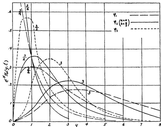
FIG. 2. Differential straggling functions for an electron that loses energy by radiation only. The numbers attached to the curves are thickness in radiation units.  $y = \ln(E_0/E)$ .
