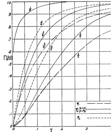
FIG. 3. Integral straggling functions for an electron that loses energy by radiation only. The numbers attached to the curves are thicknesses in radiation units.  $y = \ln(E_0/E)$ .
