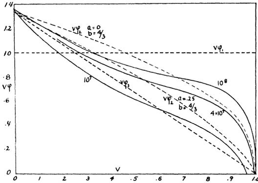
FIG. 1. The approximate expressions for the radiative cross section given by Eqs. (12) are plotted as dotted lines and the correct expressions for various energies in air as solid lines.
