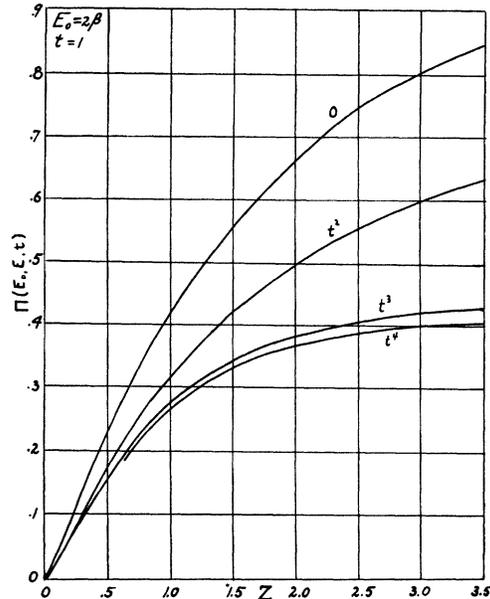
FIG. 4. Illustrating the effect of including higher powers of  $t$  in the integral straggling function  $\Pi_{\beta}(E_0, E, t)$ , for  $E_0 = 2\beta$ ,  $t = 1$  and  $\varphi(v) = \varphi_1(v)$ . The curve marked 0 corresponds to taking only the constant term  $c_0(s)$  in the series (26), that marked  $t^2$  corresponds to taking  $c_0(s) + c_1(s)t^2$ , etc.  $Z = \ln(E_0 - \beta t/E)$ . For  $E_0 = 2\beta$ ,  $t = 1$ ,  $Z = \ln \beta/E$ .
