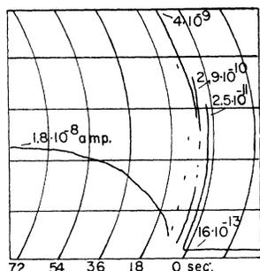
FIG. 4. Rise of the photo-current in CdS at room temperature (curves taken with stepwise decrease of input resistances).
