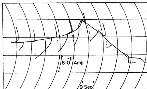
FIG. 6. Curves showing that the building up of stationary positive space charges is independent of the electric field to the first approximation. Continuous curve: Field applied at the CdS crystal during irradiation. Interrupted curve: Field periodically removed during irradiation.
