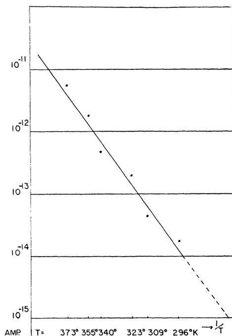
FIG. 2. Temperature dependence of the conductivity of CdS.
