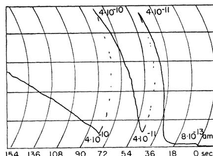
FIG. 3. Rise of the photo-current in CdS at liquid air temperature (curves taken with stepwise decrease of input resistances).
