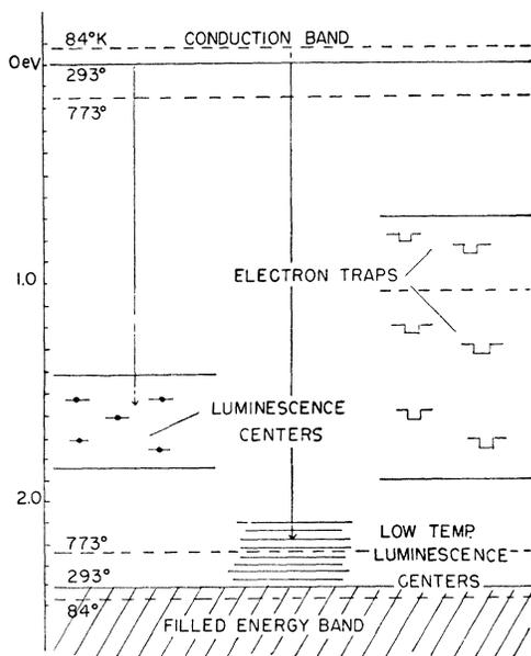
FIG. 1. Band scheme of CdS.
