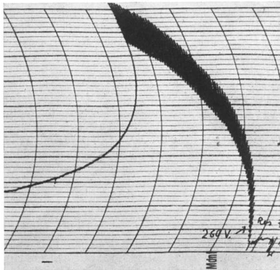
FIG. 5. Current produced in CdS by periodical irradiation with  $\gamma$ -rays.
