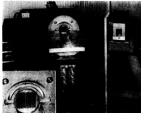
FIG. 1. Comparison of new and old lead collimators for the two-meter focusing curved-crystal gamma-ray spectrometer. To indicate the scale, a horizontal one-foot rule can be seen at the back of the lead shielding on the new collimator. The cylindrical multicellular counter and the upper half of the lead shields that cover it have been removed. The semicircular cavity that can be seen in the end of the first circular lead shield is provided to accommodate the battery of anticoincidence counters which in operation are situated above the multicellular counter to protect it from cosmic rays. A meter stick stands vertically near the old collimator which is at the right. Both collimators are 30 inches long. The insert is an enlarged view of the exit end of the new collimator, the thicker ends of the tapering lead partitions being visible.
