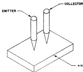
FIG. 1. Arrangement of electrodes.
