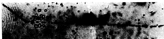
FIG. 1. \text{Li}^6 disintegration by a neutron from a mixed Po+Be source. R_\alpha = 17.5\mu , R_T = 86.2\mu , and \theta = 149^\circ . Approximate range energy curves and Q = 4.64 Mev give a neutron energy of 4.6 Mev.
