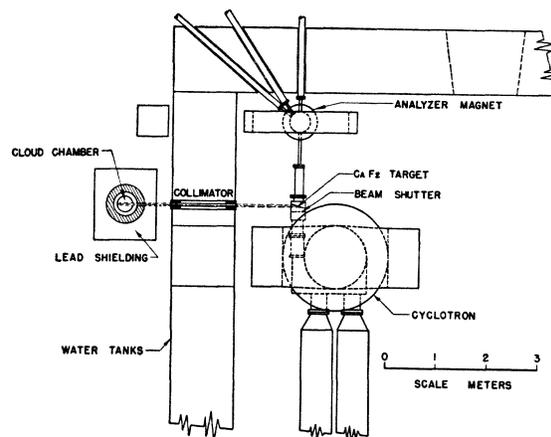
FIG. 4. A schematic diagram showing the location of the cloud chamber with respect to the cyclotron. A 1-in. hole through lead plugs in the water tanks surrounding the cyclotron collimates the radiation from the target.
