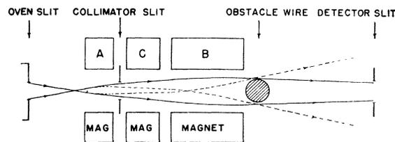
FIG. 4. Diagram of the essentials of an atomic beam system illustrating the effect of insufficient deflecting power.
