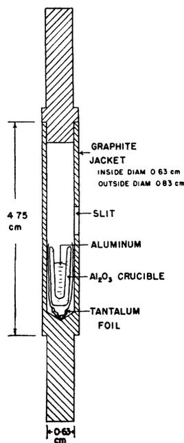
FIG. 3. Oven for generating a beam of aluminum atoms.
