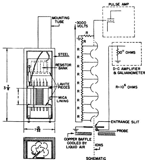
FIG. 2. Electron multiplier and circuit.
