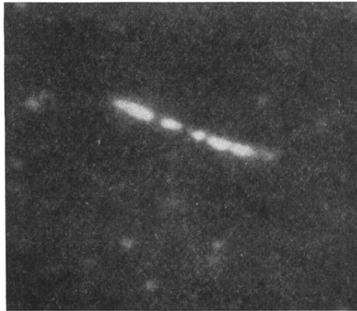
FIG. 1. Typical tracks each produced by one fission fragment in one of the U^{238} monitoring foils.
