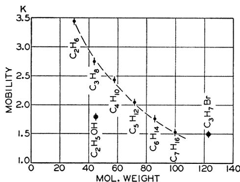
FIG. 2. Mobilities of various molecular ions as a function of molecular weight.
