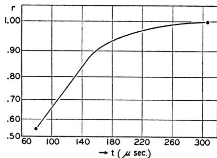
FIG. 1. Plot of  $r^2$  vs. the dead-time  $t$ , showing linear relation up to  $r=0.9$ .
