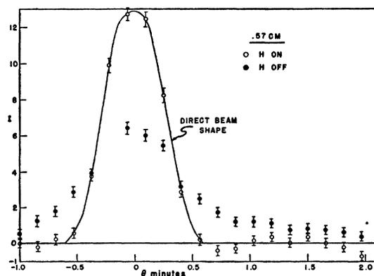
FIG. 3. Neutron distribution after passage through a magnetized ("H on") and an unmagnetized ("H off") iron block. The smooth curve is the same curve as shown in Fig. 2, adjusted by an intensity scale factor.
