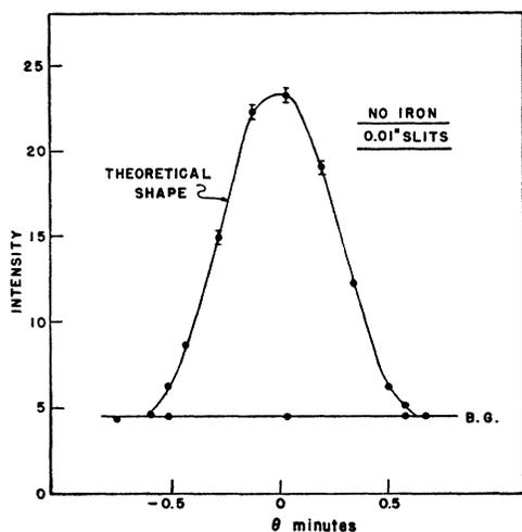
FIG. 2. Angular distribution of neutrons in the beam of Fig. 1 as detected with a 0.01-in. counter slit with no iron block in the beam.
