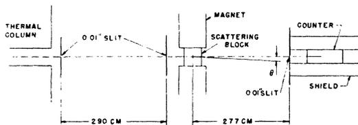
FIG. 1. Apparatus for measurement of magnetic small-angle scattering using slit geometry.
