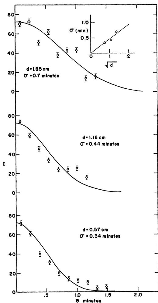
FIG. 4. Experimental neutron distributions for different block thicknesses,  $d$ , compared to curves calculated on the assumption that each part of the direct beam is spread into a Gaussian of width  $\sigma$ . The variation of the  $\sigma$  used for each block with  $d$  is also shown.
