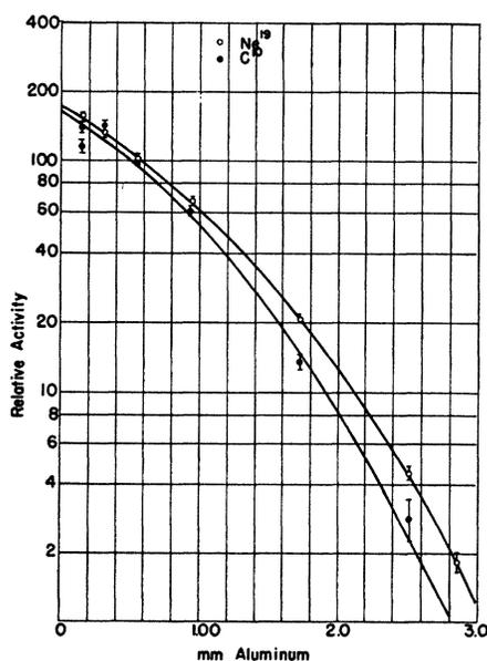
FIG. 6. Positron absorption curves for  $Ne^{19}$  and  $C^{10}$ . The data of Fig. 5 are replotted with  $\gamma$ -ray backgrounds subtracted. The abscissae have been corrected for the counter window and the inspection cell window.
