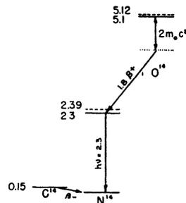
FIG. 12. Energy level diagram of  $O^{14}$ ,  $N^{14}$ , and  $C^{14}$ . The energies are given in Mev. The dashed lines represent calculated values.
