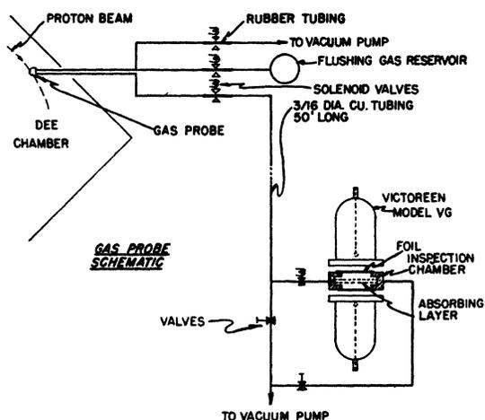
FIG. 2. Schematic drawing of the gas probe system, showing the probe, control valves, and counting arrangement.
