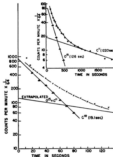
FIG. 4. Decay of radioactive gases from bombardment of  $CaF_2$ ,  $B^{10}F_3$  by protons. The gases have been trapped by ascarite. The upper graph shows the longer period activities, the lower graph shows the  $C^{10}$  decay.
