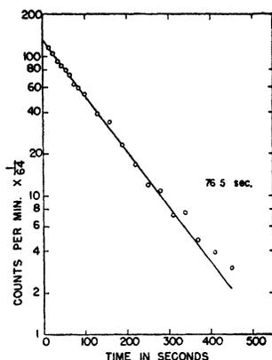
FIG. 9. Decay of radioactive gases produced by bombardment of KSCN by protons and trapped by  $\text{CaCl}_2$ .
