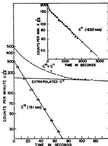
FIG. 3. Decay of radioactive gases from bombardment of boron by protons. The upper graph shows the  $C^{11}$  decay, and the lower graph shows the  $C^{10}$  decay.
