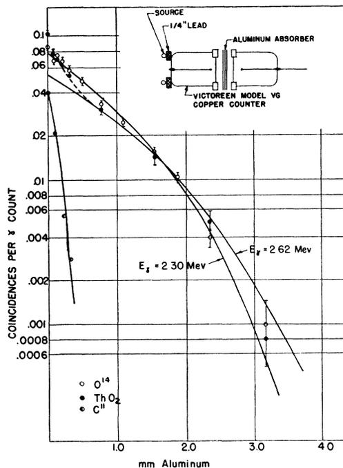
FIG. 11. Coincidence absorption measurements of gamma-radiations of  $O^{14}$ . The insert shows the counting arrangement.
