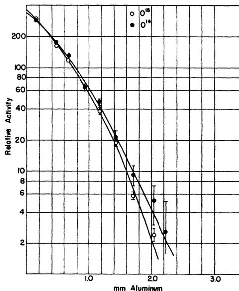
FIG. 10. Positron absorption curve for  $\text{O}^{14}$  and  $\text{O}^{16}$ . The gamma-ray backgrounds have been subtracted.
