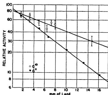
FIG. 7. Absorption of gamma-radiation in lead.
