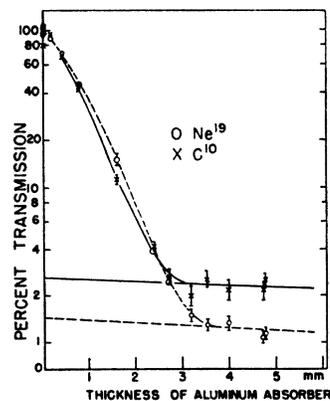
FIG. 5. Positron absorption curves for  $Ne^{19}$  and  $C^{10}$ , taken under identical geometrical conditions. The abscissae refer to added aluminum absorber.
