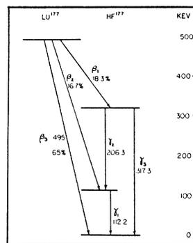
FIG. 1. Proposed decay scheme for Lu<sup>177</sup>.
