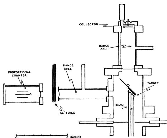
FIG. 1. Schematic diagram of bombardment chamber. The target is mounted on a Wilson seal and may be turned aside. The range cell behind the target is for measuring the energy of the deuteron beam. The range cell at right angles to the beam measures the range of the protons. An automatic foil changer between range cell and counter makes large changes of absorption possible.
