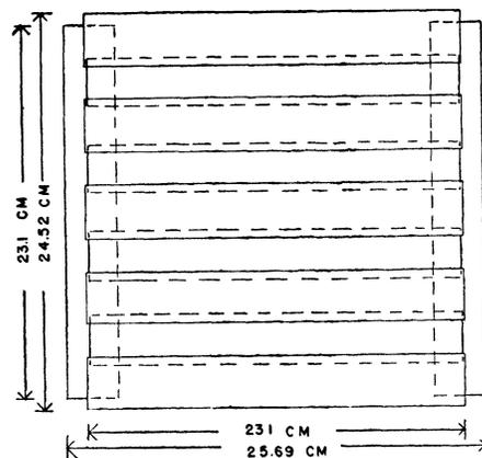
FIG. 1. Plan view of a single tray of Geiger counters. The effective dimensions of the individual counters are shown. Note that the counters overlap so that only about  $\frac{2}{3}$  of the effective area of each is utilized.
