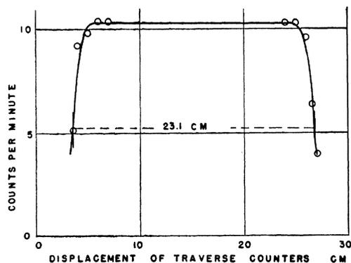
FIG. 2. Effective length of counter as determined for five counters simultaneously using the method of Street and Woodward. The shape of the curve depends on the diameter of the counters, the effective length being given by the distance between half-maximum points.
