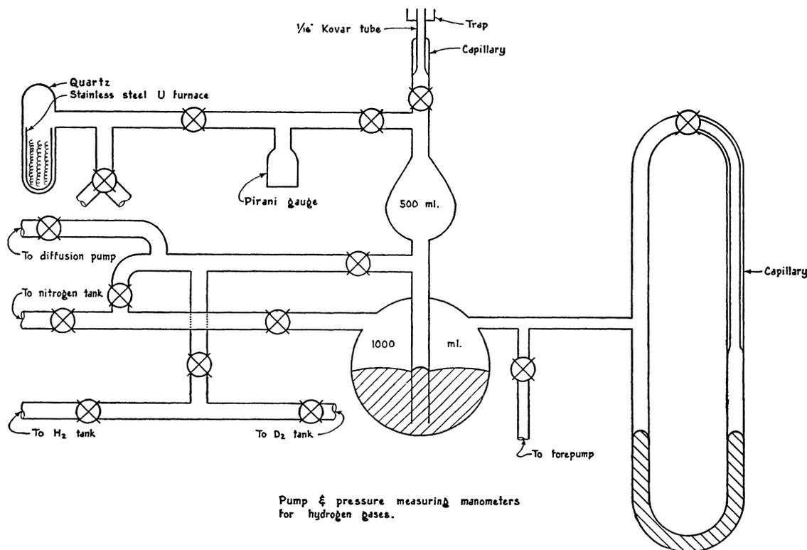
FIG. 1. Tritium storage and gas handling system.
