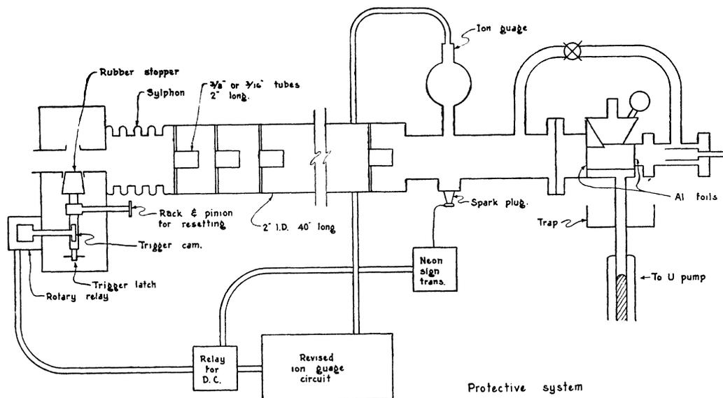
FIG. 2. Gas impedance tube and circuits for tritium recovery in case of foil breakage on target.
