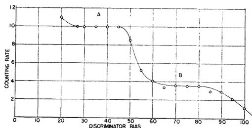
Fig. 1. Typical curve of the counting rate as a function of the discriminator bias showing the relative size of the scattered proton pulses and recoil helium pulses which entered the proportional counter.
