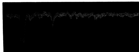
FIG. 15. Presence of first sound detected by vibration microphone ( T=2.09^{\circ}\text{K} ). Note short time delay due to higher velocity.
