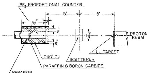
FIG. 1. Geometry used in scattering experiments.
