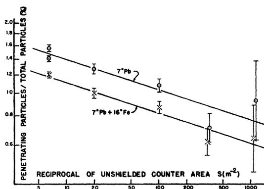
FIG. 4.  $R$  versus  $1/S$ , for penetrating particles capable of penetrating 7" Pb and 7" Pb + 16" Fe.
