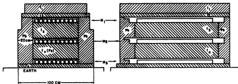
FIG. 1. Arrangement of shielded counters and absorbers.
