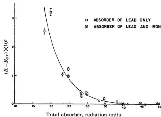
FIG. 7. The part of R not due to penetrating particles, plotted versus total absorber thickness, measured in radiation units.
