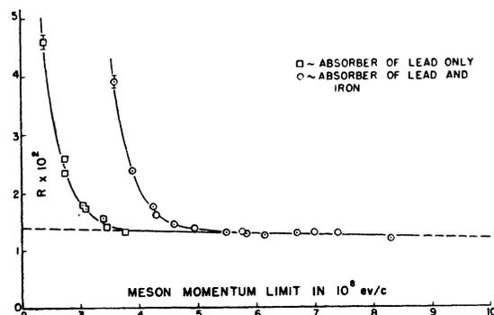
FIG. 6.  $R$  versus total absorber thickness, expressed in terms of the meson momentum limit. The points enclosed in squares refer to lead thicknesses from 4 to 8 inches. The least absorber including iron was 2 inches lead plus 6 inches iron.
