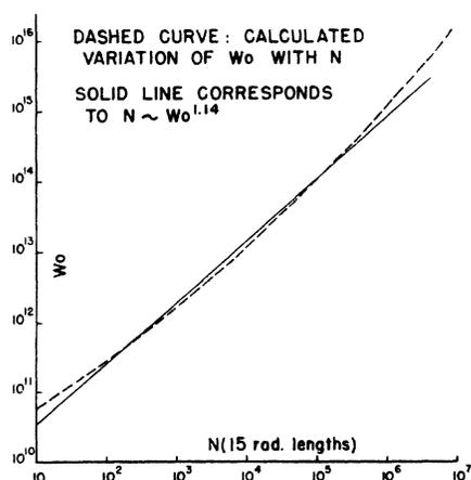
FIG. 5. Numbers  $N$  of electrons generated after 15 radiation lengths in air by a photon of energy  $W_0$ .
