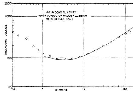
FIG. 5. Comparison of experimental points and theoretical curve for coaxial breakdown.
