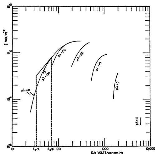
FIG. 1. Ionization coefficient (ionizations/volt<sup>2</sup>), as a function of  $E/p$  (volts/cm-mm Hg) and  $p\lambda$  (mm Hg-cm). The straight-line approximation used to compute coaxial breakdown agrees with numerical integration using the correct value to within one percent.
