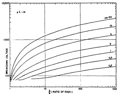
FIG. 4. Breakdown voltage between coaxial cylinders as a function of  $b/a$ , ratio of outer conductor radius  $b$  to inner conductor radius  $a$ , and  $p\lambda$  (mm Hg-cm). This family of curves applies for  $p\lambda = \infty$ . A separate family is required for each value of  $p\lambda$ , for a complete set of curves.
