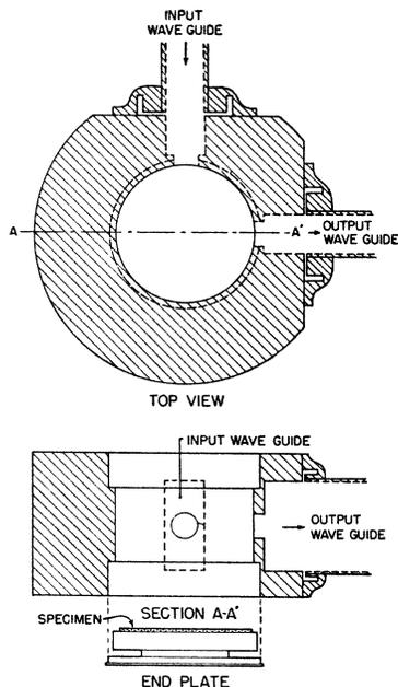
FIG. 2. Wave-guide assembly with fixed coupling holes. End plate shown retracted.
