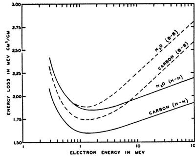
FIG. 5. The theoretical ionization loss for electrons in carbon and H<sub>2</sub>O. The Halpern-Hall loss is shown by the solid lines, the Bethe-Bloch loss by the dotted lines.
