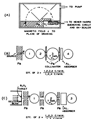
FIG. 1. (A) The beta-ray spectrometer for determination of the primary ionization in the 0.2–0.75 Mev range. (B) The coincidence apparatus for measurements at higher energies. (C) Revised coincidence arrangement using B<sup>12</sup> beta-spectrum produced by deuteron bombardment of B<sup>11</sup>.
