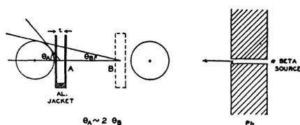
FIG. 6. Schematic diagram of apparatus for investigation of relative stopping powers.  $\theta$  represents the maximum angle through which an electron may be scattered and still record a coincidence.
