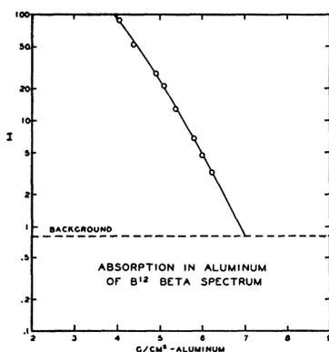
FIG. 7. Logarithmic plot of the higher energy points from Fig. 3 for determination of the end point of the  $B^{12}$  beta-spectrum.
