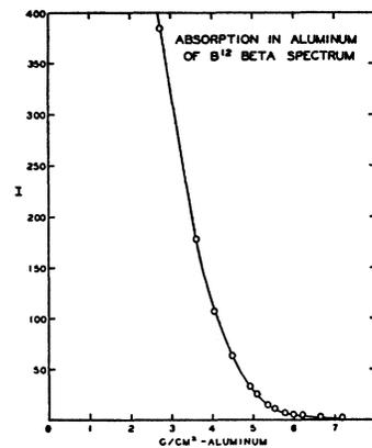
FIG. 3. Absorption in aluminum of beta-rays from  $B^{12}$ . See Fig. 7 for end-point determination.
