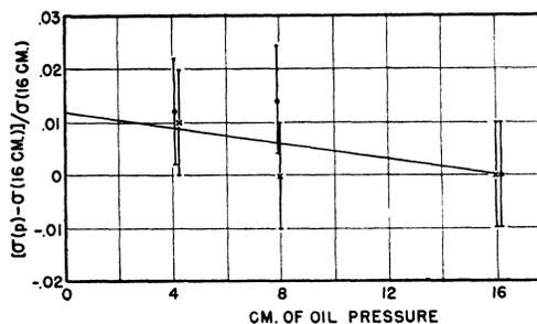
FIG. 2. The fractional change in the measured cross section for scattering through  $8^\circ$  of 2.42-Mev protons as a function of the pressure,  $p$ , of the hydrogen filling the scattering chamber.
