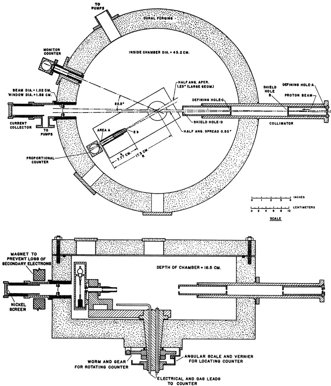
FIG. 1. Plan and elevation of the scattering chamber. Upper figure is a section through the plane of the incident beam and the beam scattered through the analyzer slits and detectors. Elevation is a section through the incident beam. The moveable analyzer slits and detector are not in the same position in the two sections.
