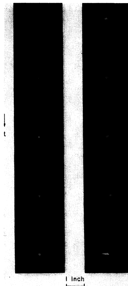
FIG. 5. Consecutive frames taken with Fastex Camera located in the plane of the orbit. The center of the orbit is to the right of the spot. The r-f was turned off before peak magnetic field (after frame 8). The orbit contracts (frame 9) and then expands, moving to the left in the final frame.
