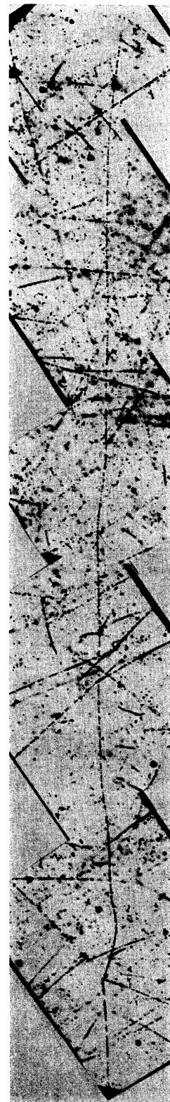
FIG. 22. Track of a negative meson (mass = 300 me) in Eastman NTB emulsion. Range in emulsion 400 microns. Exposure made on University of California cyclotron.
