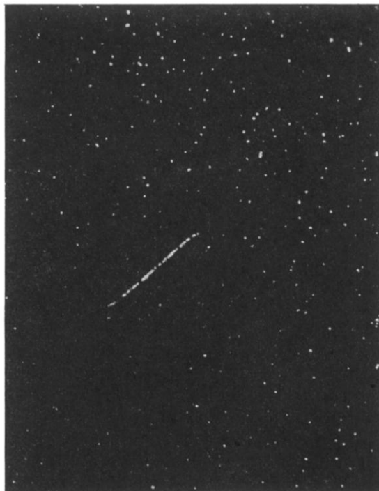
FIG. 19. Track of U^{235} fission on Eastman NTC emulsion, obtained by impregnating emulsion with uranium acetate and bombarding with slow neutrons.
