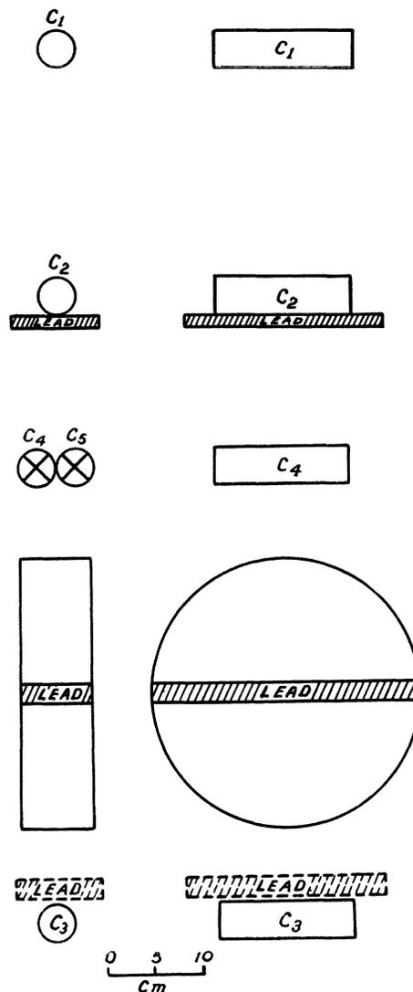
FIG. 3. Side and front view of the arrangement of counters, etc., with respect to the Wilson chamber.  $C_4$  and  $C_5$  are the counters connected to the anticoincidence circuit. The lower lead block shown dotted was removed in some of the observations.
