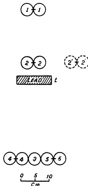
FIG. 1. Arrangement of counters for determining the shower maximum for more than one particle and more than two particles in lead. Each of the counters 1, 2, 4, and 5 are, in fact, two counters joined in parallel.
