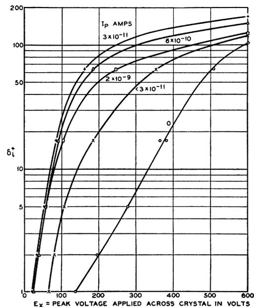
FIG. 9. Peak positive yield as a function of various values of superimposed steady bombarding current.
