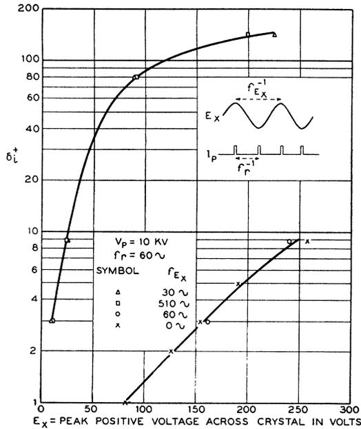
FIG. 8. Effect of space-charge neutralization on peak positive yield.
