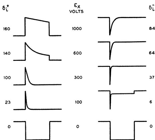
FIG. 5. Variation of observed pulse shapes with crystal voltage  $E_x \cdot V_p = 10$  kv,  $i_p = 0.5 \mu\text{amp.}$ , pulse length =  $5 \mu\text{sec.}$
