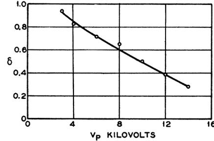
FIG. 4. External secondary electron emission from gold electrode.
