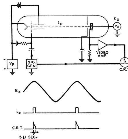
FIG. 3. Experimental schematic and time relationships.
