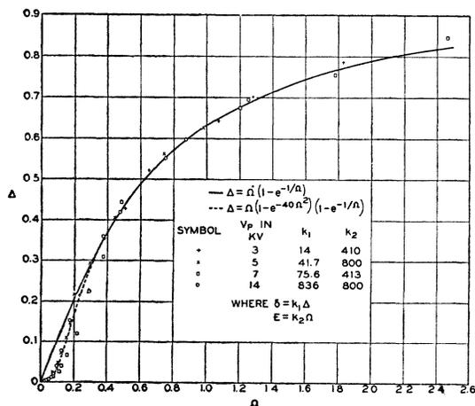
FIG. 10. Comparison of theoretical yield curve with experimental results.
