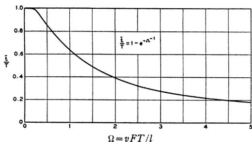
FIG. 11. Theoretical variation of probable "transit" time with electron range.
