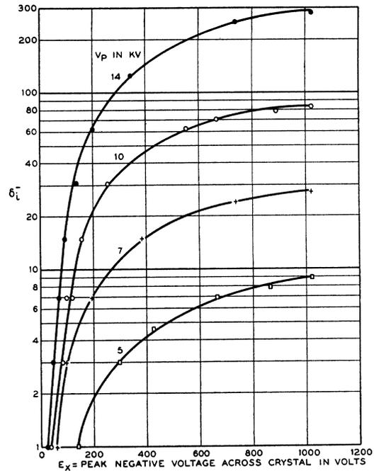
FIG. 7. Peak negative yield for space-charge neutralized crystal.
