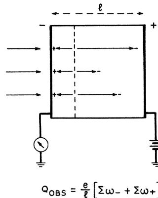
FIG. 1. Illustration of principle of bombardment induced conductivity.
