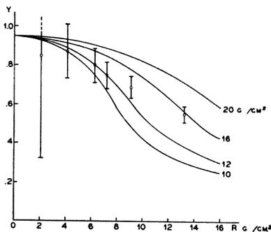
FIG. 2. The yield  $Y$  as a function of the absorber radius with range as the parameter.
