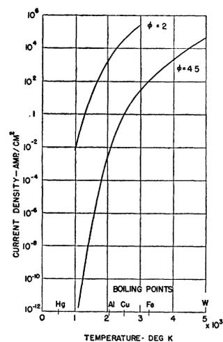
FIG. 8. Thermionic emission curves.
