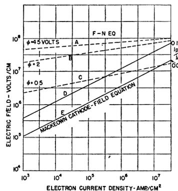
FIG. 9. Relations between cathode field and current density (electrical quantities in practical units).
