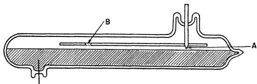
FIG. 1. Tube for mercury arc studies.
