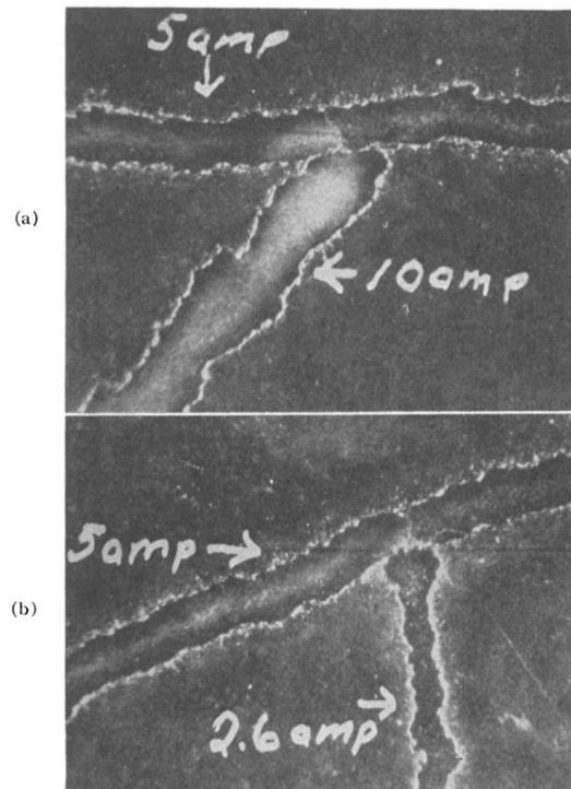
FIG. 7. Cathode tracks on tungsten.
