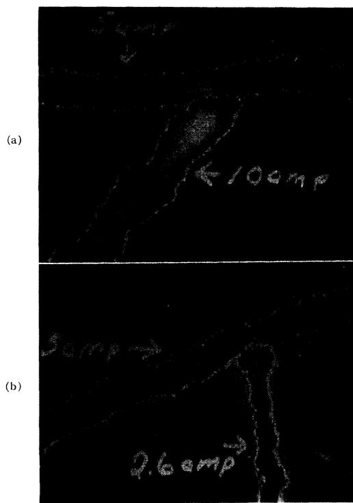
FIG. 7. Cathode tracks on tungsten.
