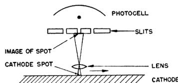
FIG. 3. Optical system for scanning the mercury cathode spot.
