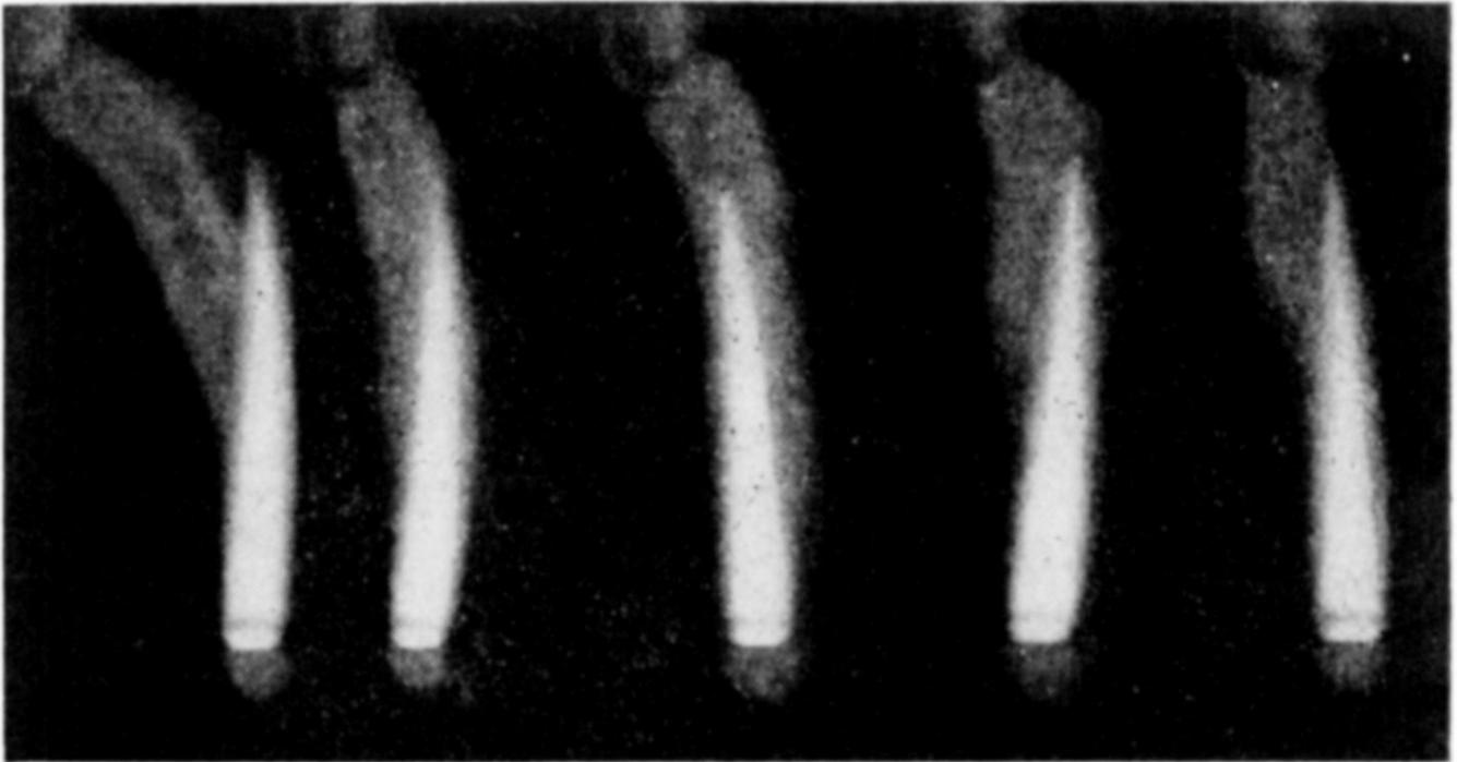
FIG. 2. Photograph of five individual sparks showing cathode mercury vapor jets. The mercury pool (cathode) is at the bottom. (Retouched.)
