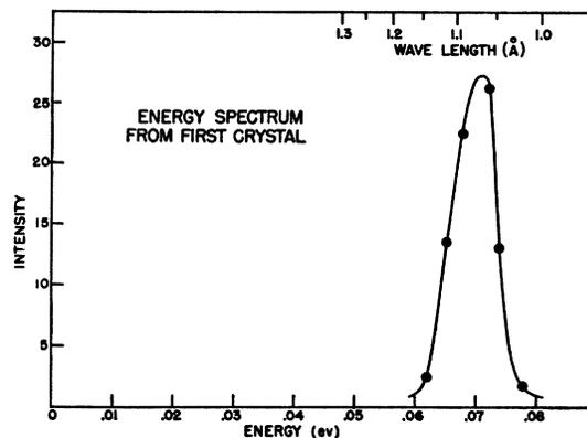
FIG. 2. Energy and wave-length distribution of neutrons reflected from monochromating crystal.
