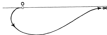
FIG. 2. The contour which defines the Hankel function of the first kind.
