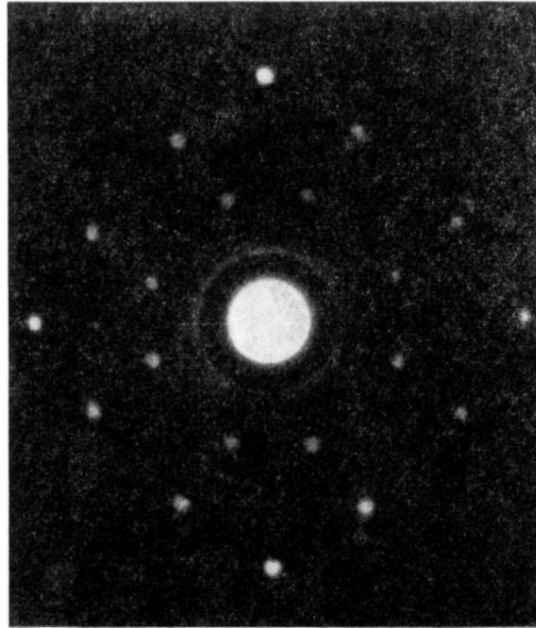
FIG. 1. Laue photograph showing neutron diffraction by NaCl.
