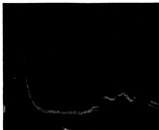
FIG. 6. This oscilloscope photograph shows the ion current to the probe as a function of the time. The markers are at 10-microsecond intervals. The peak on the left is the arc pulse, and those on the right represent the effect of the phase oscillations. There are three modulation cycles in this photograph.
