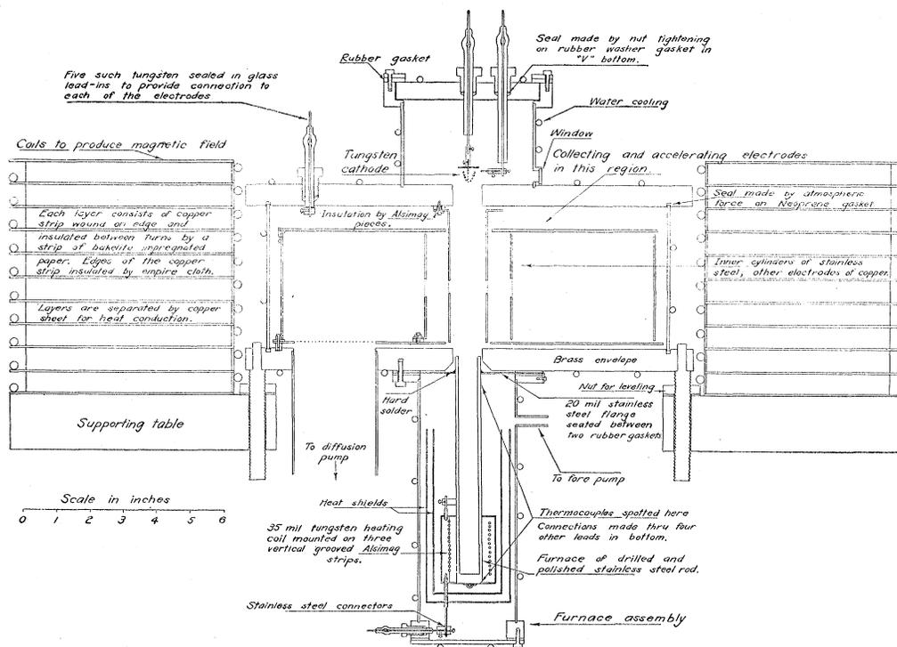
FIG. 9. Apparatus used in the investigation of the radial magnetic separator showing typical electrode arrangement.
