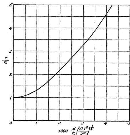
FIG. 3. Natural divergence of a beam of circular cross section in which only radial forces are assumed.  $r_0$  is the original radius;  $r$  the final radius;  $d$ , distance traveled;  $i$ , total current;  $V$ , initial voltage; and  $A$ , the atomic weight of the particles. Practical units used throughout.
