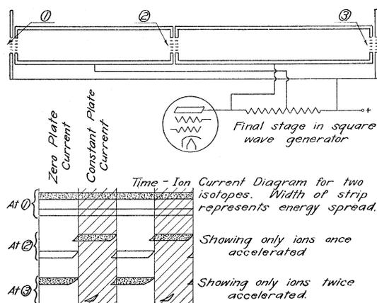
FIG. 8. Modulator and its principle of operation.
