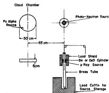
FIG. 1. Experimental arrangement of source and cloud chamber for the measurement of photo-neutron energies.
